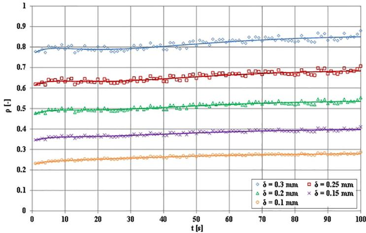
**Figure 11.** Spectral radius  $\rho$  of the stability matrix  $[a_{\text{stabil}}]$  (formula (26)) for different ceramics thickness  $\delta$  for undisturbed (solid line) and disturbed (markers) measurement of temperature  $T_g$
