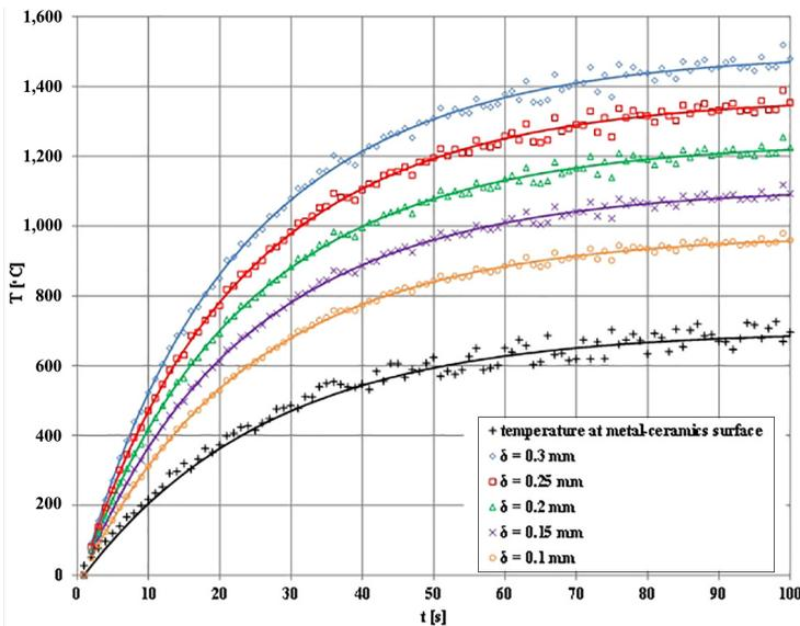
**Figure 12.** Influence of ceramics thickness on temperature on the outer ceramics surface for undisturbed (solid line) and disturbed (markers) measurement of temperature  $T_g$
