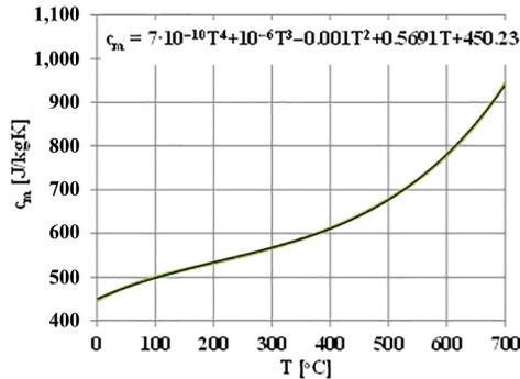
thermophysical parameters as a function of temperature. The spectral radius of the stability matrix turned out to be less than 1.0 to a depth of about 4 mm from the outer surface. Placing thermocouples at points where the spectral radius reaches the minimum is of great practical importance, as the smaller the value of the spectral radius, the greater the suppression of temperature measurement errors.
