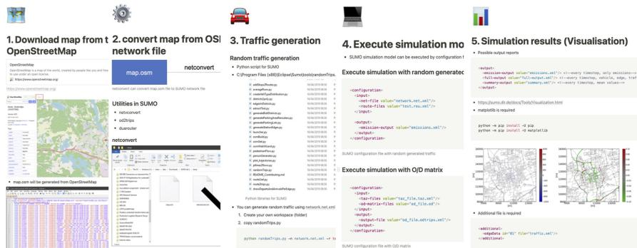
**Note(s):** (1) Export a map from the OpenStreetMap (OSM); (2) Convert the map from OSM to SUMO network file; (3) Generate traffic flows; (4) Execute the simulation model; (5) Analyse and visualise simulation results
