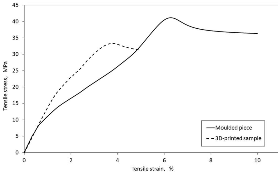
**Figure 8** Sample runs during the bend test for samples made in the injection moulding technology and samples made in the FFF technology
