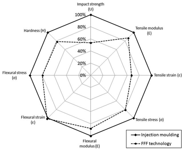
Deformation of the printed sample during the tensile strength test is 67 per cent, while during the bend test, it is 101.5 per cent of the values obtained for injection moulded samples. Hardness and impact strength of the printed samples are considerably lower and ranges between 50 and 80 per cent in comparison with the solid ABS moulded pieces.
