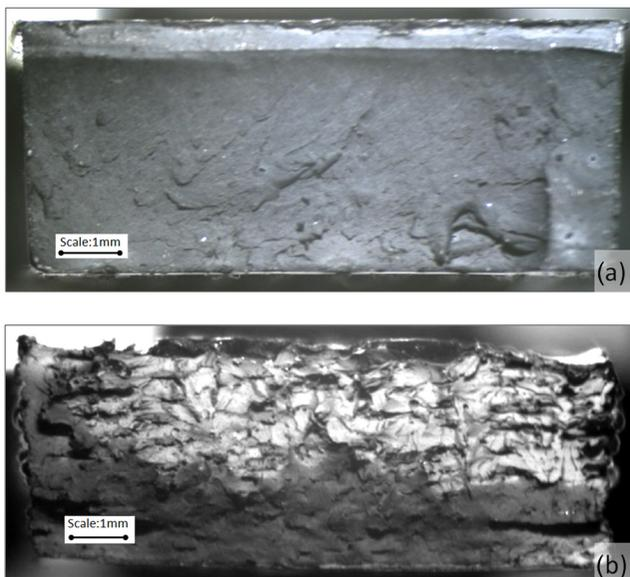
**Figure 11** Difference in material structure of the samples (fractures) of the tested technologies: a) injection moulding, b) FFF technology
