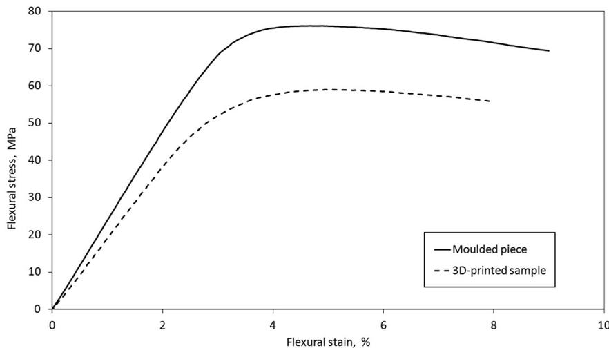
**Table II** Results of mechanical properties tests for samples made by injection moulding and samples made in the FFF technology
