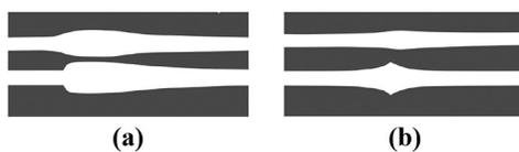
**Figure 19** Illustration of experimental (top) width and simulation (bottom) of flow rate from results for 0.3 mm layer height and (a) acceleration region for  $K_{LA} = 0$  and (b) deceleration region for  $K_{LA} = 0.0$ . Edges traced using the software Inkscape for image clarity
