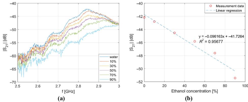
**Figure 7** The transmittance ( $|S_{21}|$ ) of the second, ring resonator for the frequency range from 2 GHz to 3.2 GHz in a function of the various volumetric concentration of ethanol in deionized water (a) and the changes of the  $|S_{21}|$  parameter for different concentrations of ethanol at  $f = 2.57$  GHz (b)
