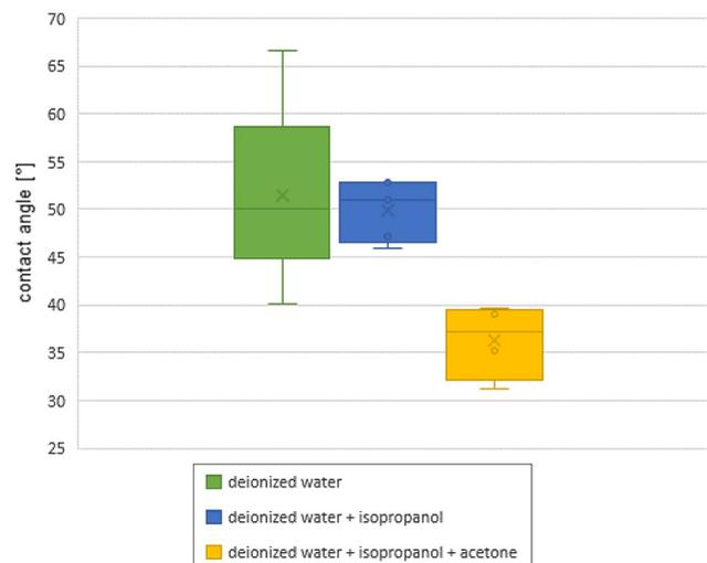
As a result, the substrates were cleaned in the deionized water for 30 min in the ultrasonic washer Branson 8210 at room temperature. After drying, the substrates were back again placed in the ultrasonic washer in the isopropanol for 30 min at room temperature.
