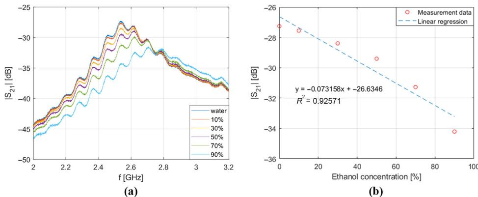
dielectric losses of the DI water around this frequency. The main principle of operation of the described microwave sensor was the shift in resonance frequency for various liquids introduced to the microchannel. The solution of the different ethanol concentrations in deionized water was introduced as a test sample because of the high difference between the dielectric constant of DI water and ethanol.
