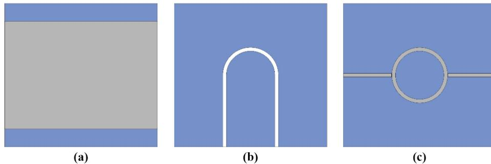
The microchannel was placed in two inner layers of the substrate (layers 2 and 3, Figure 2b). The microwave circuit was deposited on the upper layer of the substrate with the use of the ink-jet printer. The ground plane was deposited on the bottom of the module, and this time, because of cost savings, a fast version of the screen printing method was used (layer 1). Furthermore, each layer includes pads for the clamp edge-launch SMA connectors.
