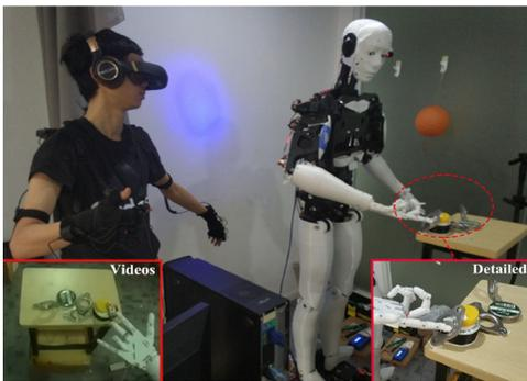
**Figure 19** Snapshots of end-effector crossing obstacles
